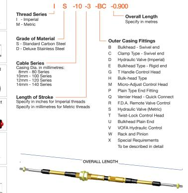
Therefore a cable IS-10-3-BC-0.900 is a 900mm long 100 Series assembly with 3"stroke, bulkhead fitted at the input end and clamp type fitted at the output end, made from standard grade material and Imperial thread sizes.
